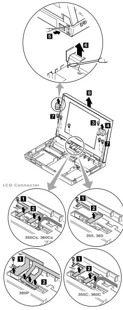
When replacing the LCD ground-terminal screw, do not pull or push the LCD cables.
